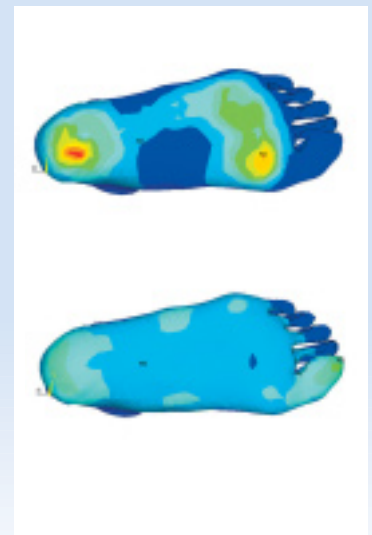
Von Mises stress distributions on the plantar surface of the foot using the flat (top) and total contact insoles (bottom)
