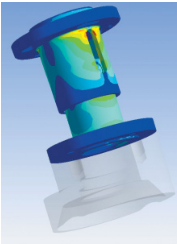
Procter & Gamble rank-and-file engineers routinely use ANSYS DesignSpace software in product development projects. Sample plots here show loads on the slotted concentric shafts of a converting machine assembly, enabling engineers to quickly evaluate the design early in development.
